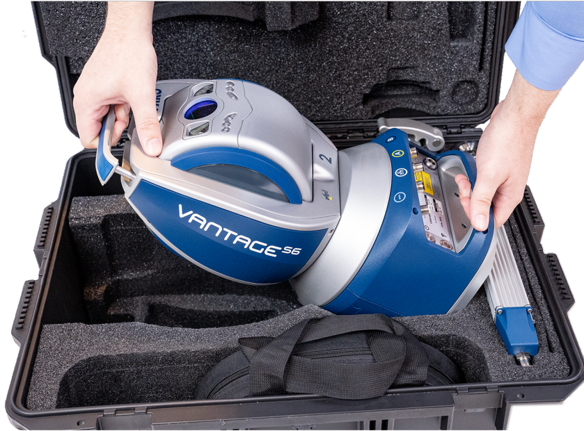
Figure 3-4 Lifting the Vantage
