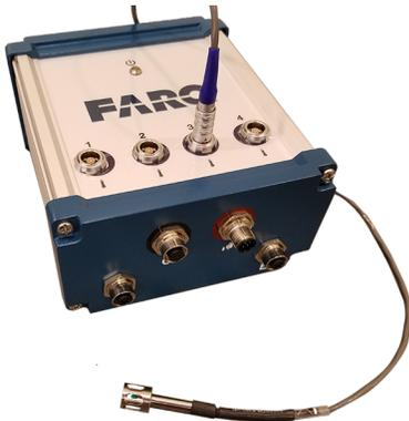
Figure 7-15 Connecting a Temperature Sensor
