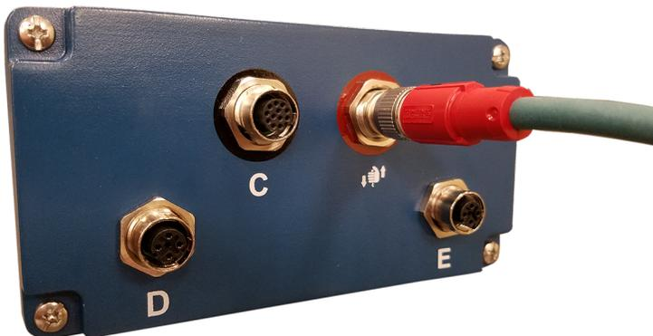
Figure 7-16 Connecting the Multi-use Integrator cable
