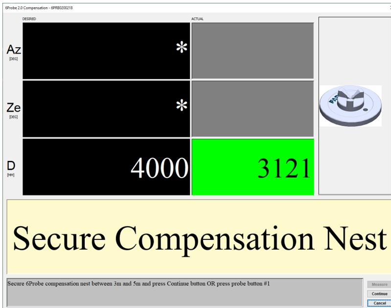
Figure 2-25 Secure the Compensation Nest
