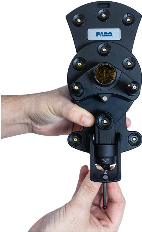
*Figure 2-14 Installing Probe*
