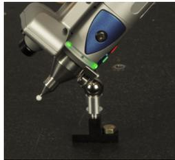
Figure 5-9 SMR Bracket Compensation
