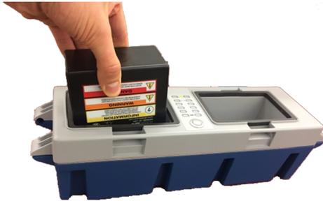
Figure 7-3 Installing the Battery Pack
