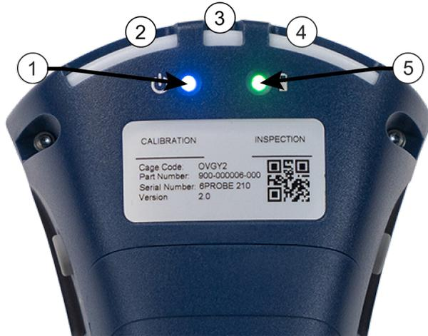
Figure 2-4 6Probe LED Indicators
