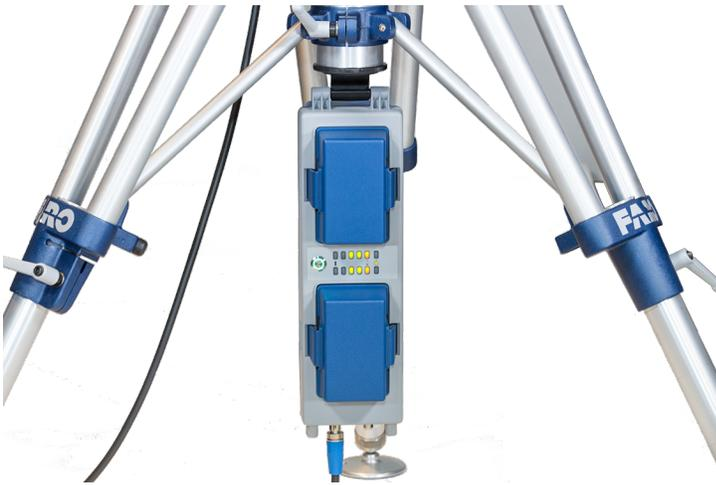
Figure 7-8 Hanging the Battery Box Kit
