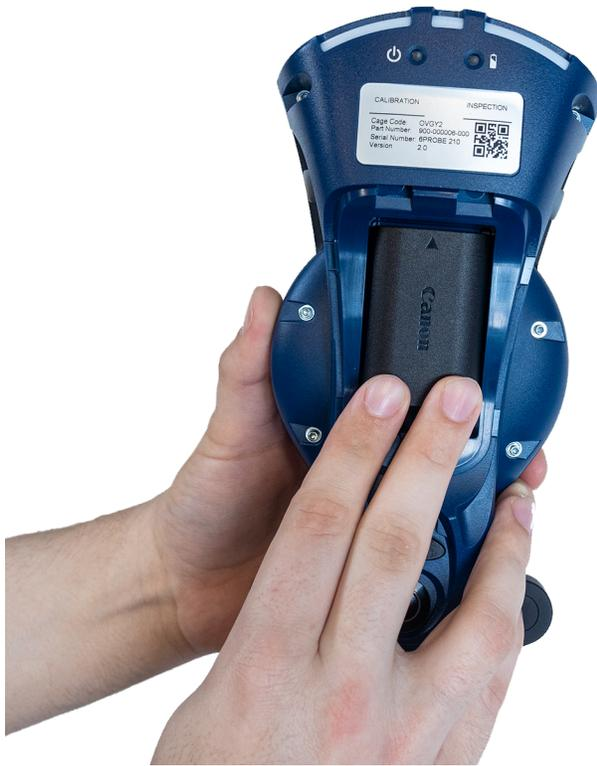
*Figure 2-10 Installing the battery*
