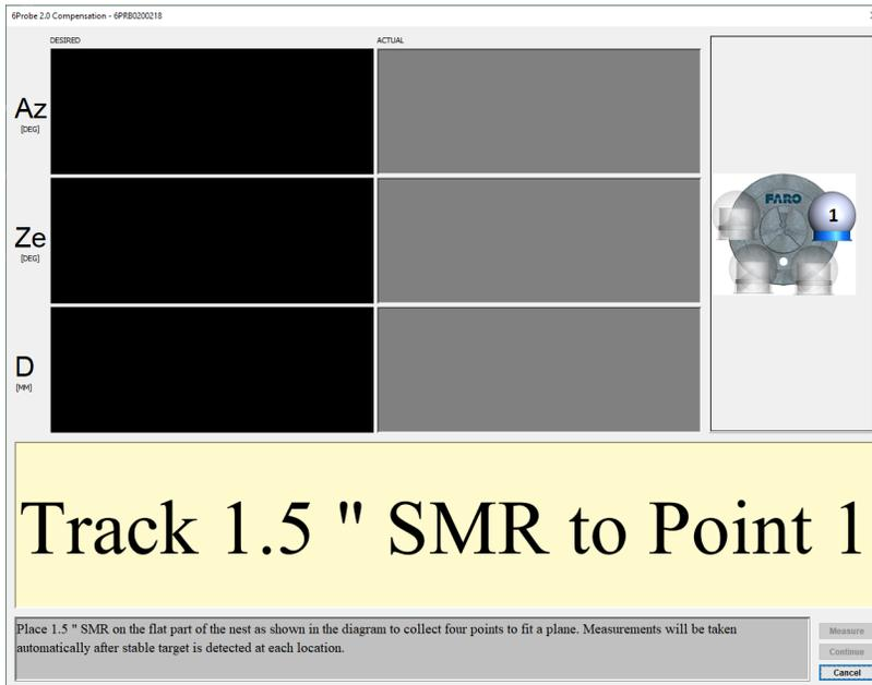
Figure 2-26 Measuring the Compensation Nest base
