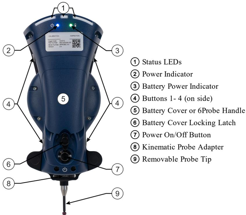
Figure 2-2 6Probe Rear View
