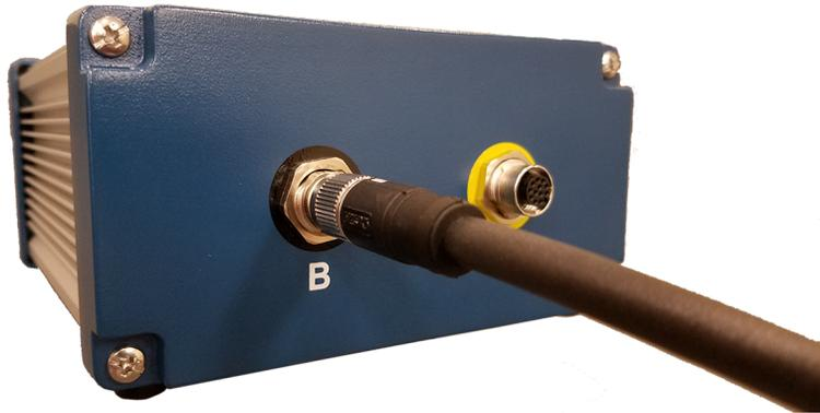
Figure 7-14 Connecting to the Laser Tracker
