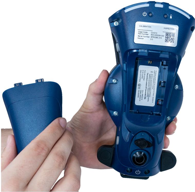
*Figure 2-9 Remove the battery cover*
