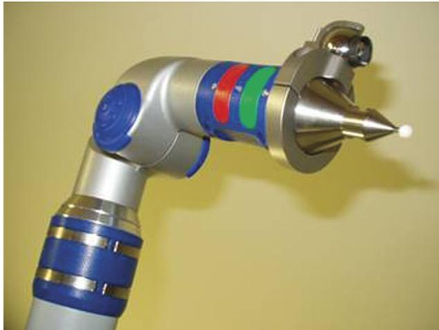
Figure 5-7 SMR FaroArm Bracket
