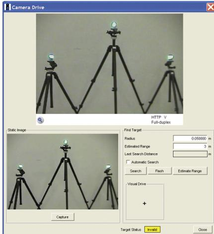
The **Zoom button** allows you to enlarge or shrink the live picture. This is helpful when working with small targets that are far away from the Laser Tracker.
