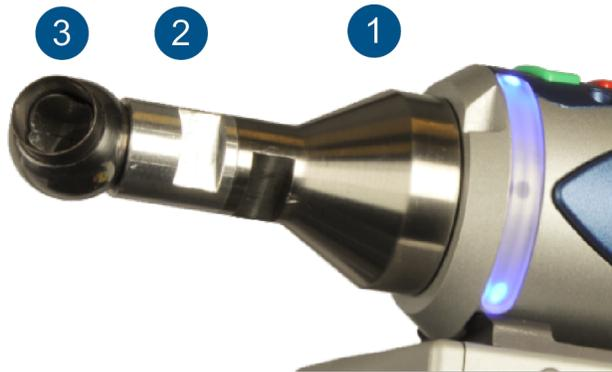
Figure 5-6 Magnetic SMR Probe Adapter
