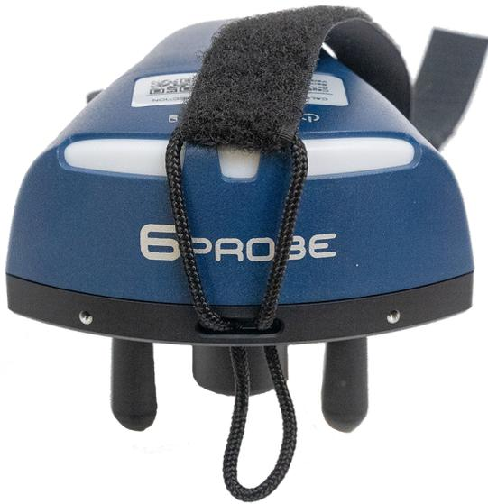
*Figure 2-36 Feed the Cord into the Slot*
