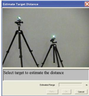
Select a target on the screen and the Laser Tracker measures the distance and switches sights. Select the target again. The two measurements are used to calculate the estimated range to the target. The estimated range improves the ability of the Laser Tracker to locate the target. If no target is found, the Laser Tracker searches for the target.
