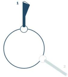
2. Digitize 11 points around the top hemisphere of the sphere with the probe pointing in position #1. Hold the handle in the same direction and orientation for every point.
