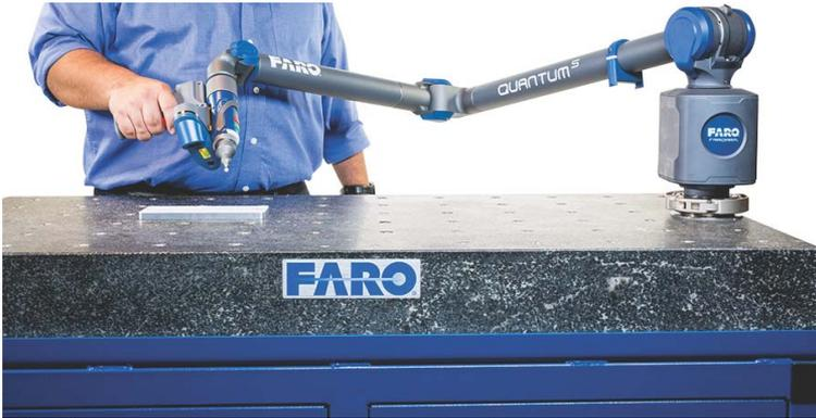
Figure 4-15 Measuring the Compensation Plate with the Laser Line Probe
