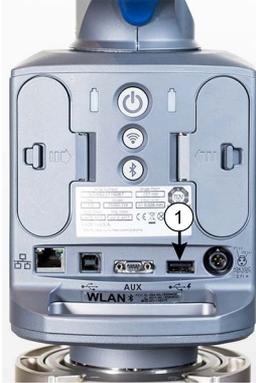
*Figure 2-21 Powered USB Port*
