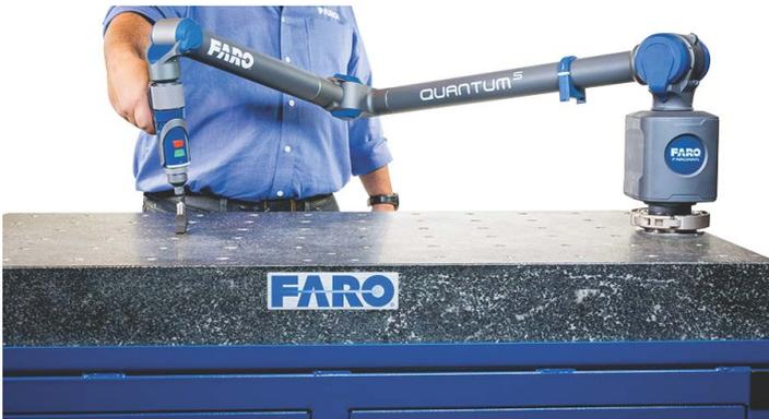
Figure 6-6 Probe Compensation
