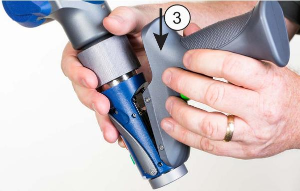
*Figure 2-11 Inserting the 7-Axis Handle*
