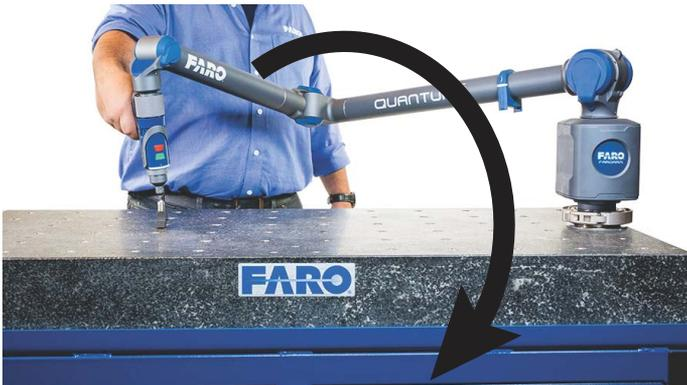
Figure 6-8 Single Point Articulating Test (SPAT)
