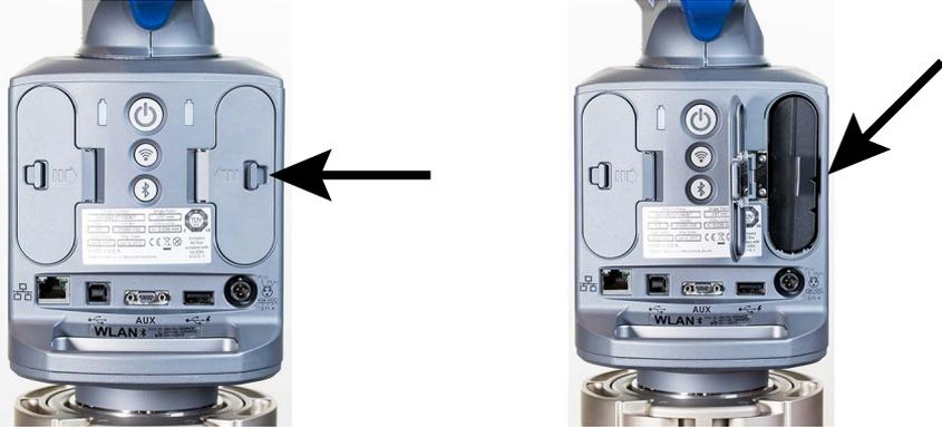
*Figure 2-19 Removing the battery pack*
