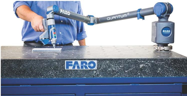
*Figure 4-14 Measuring the Compensation Plate with the Ball Probe*
