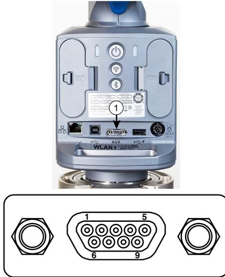
Figure 2-22 Quantum Auxiliary port
