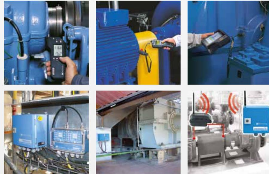
... that is, with all PRÜFTECHNIK Condition Monitoring Systems – with hand-held measurement devices, data collectors and permanently installed online systems.
