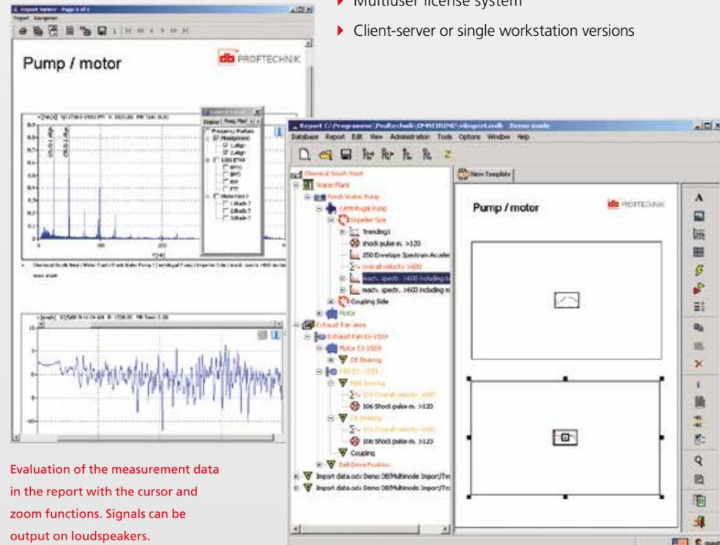
Evaluation of the measurement data in the report with the cursor and zoom functions. Signals can be output on loudspeakers.
